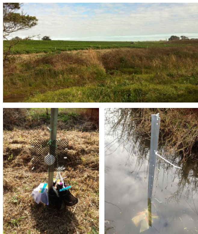
Figure 5.5 Market gardens in Western Port (top), passive samplers to assess pesticides pollution and leaf litter bags to assess functional stream health deployed in Western Port (above).
