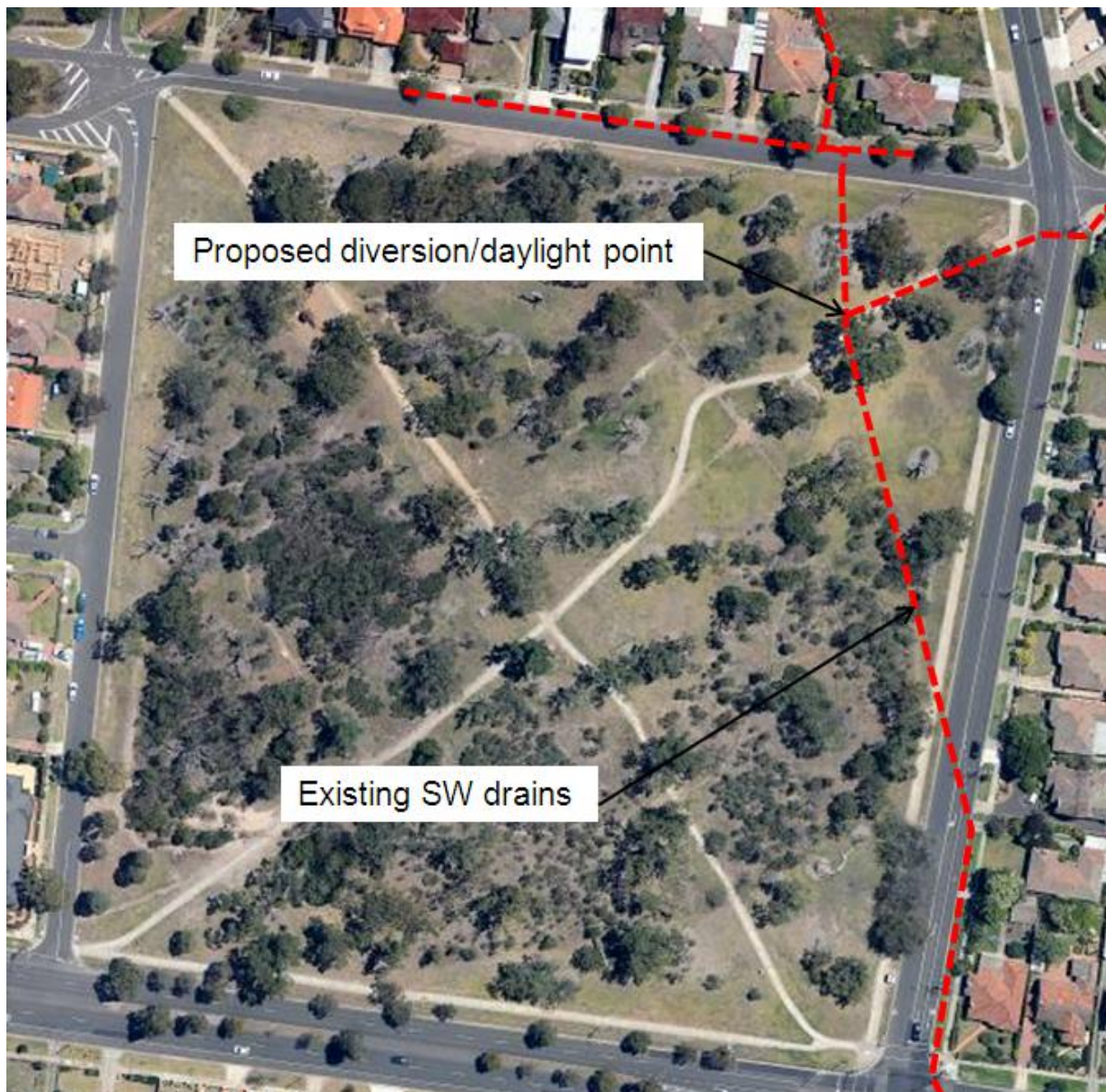
Figure 6; Napier Park site with existing drainage and proposed diversion point in north east corner (image courtesy Nearmap)
