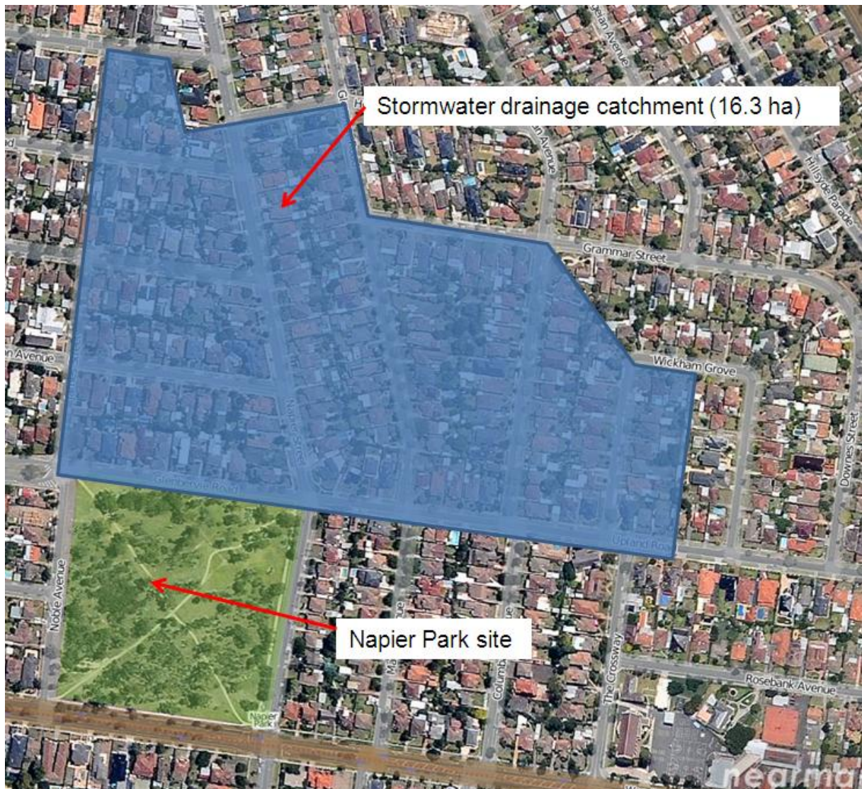
Figure 7; Contributing stormwater drainage catchment north of Napier Park
