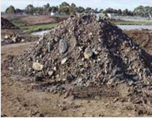
✓ Example of well graded material for filter/embedment layer.
