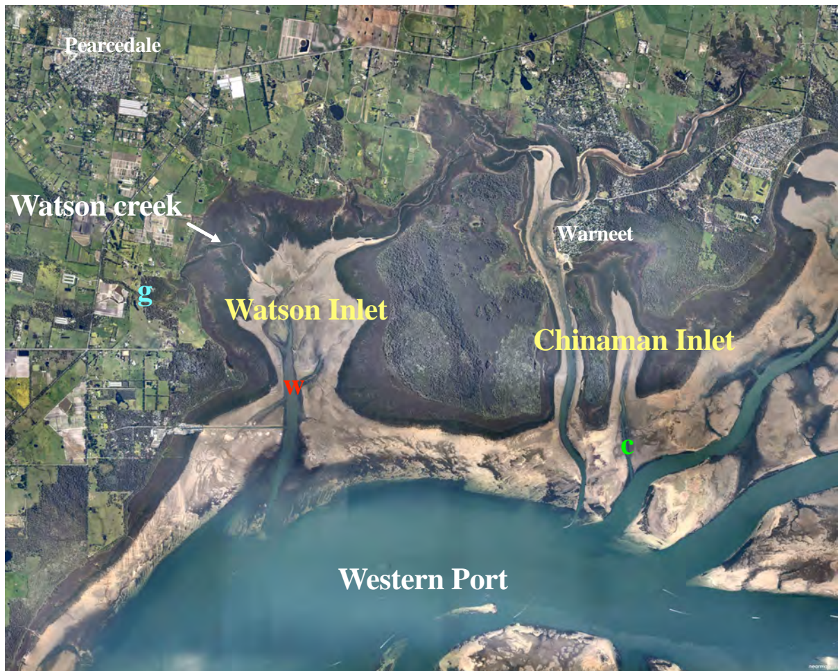
Fig. 2. Northern part of Western Port (Photo: www.nearmap.com ). Site locations and 24 h offshore survey positions for Watson and Chinaman inlets (w and c, respectively). g corresponds to the location of the gauging station on Watson Creek.
