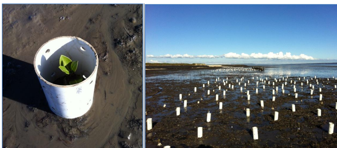
Figure 35: PVC pipe tree guard (left) randomly placed in experimental plots (right)
