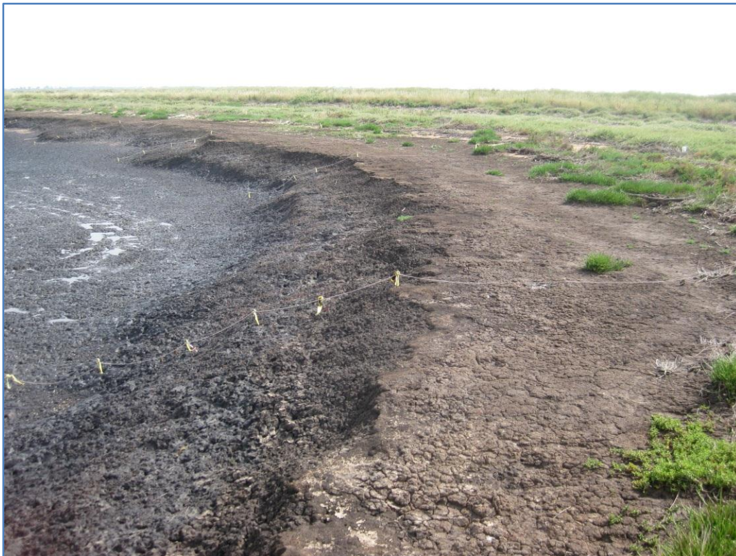
Figure 5: Erosion monitoring (erosion pins arranged in a series of transects across erosion profile) being undertaken by Tomkins and McLachlan.
