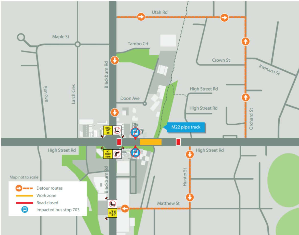
Figure 1: Work area and local traffic detour routes
