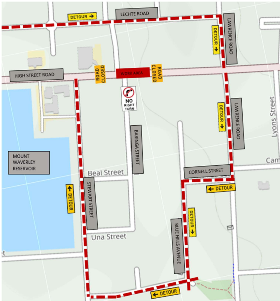
Figure 1: Work area and local traffic detour routes
