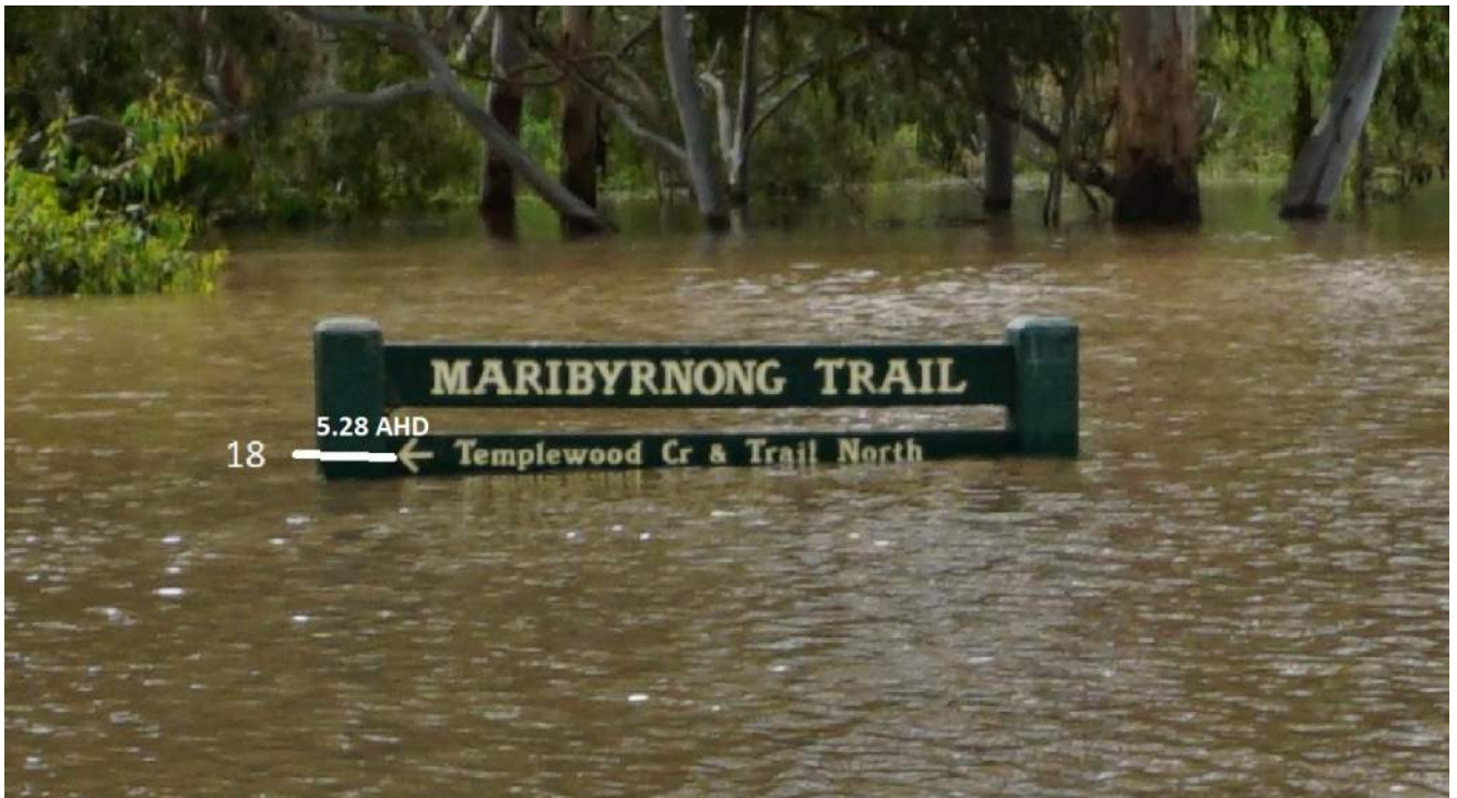
Figure 4 – Example of the flood marker surveyed with its associated horizontal position and AHD value to be utilised to help calibrate the flood model.
