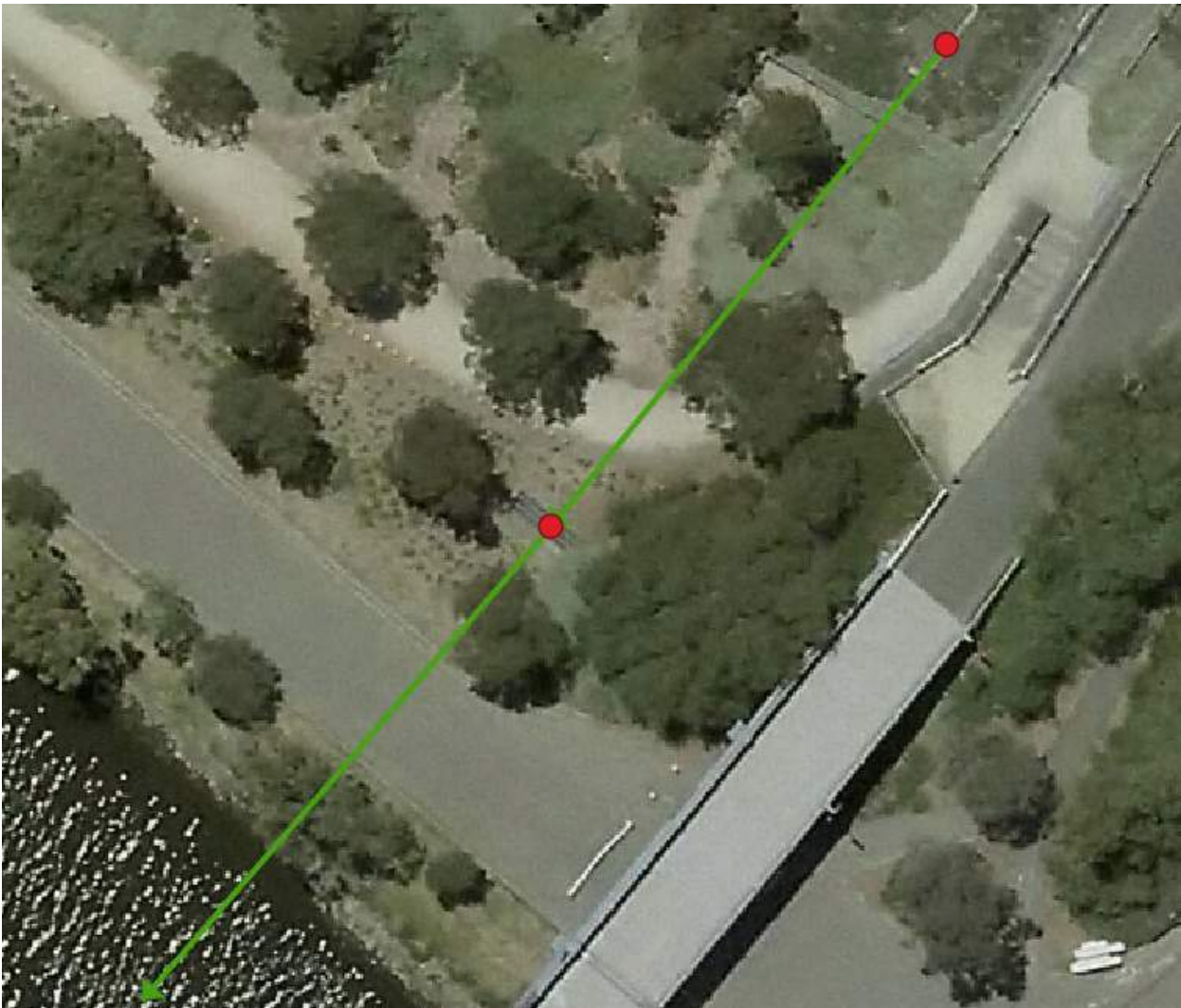
Figure 6-10: The pipe under Riverside Park levee in green, with the overflow pit and the discharge pit marked in red. The high point of the levee is marked by the dirt path.
