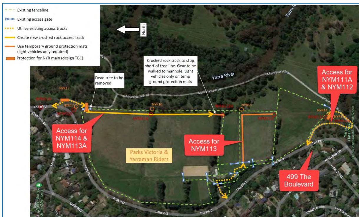
Figure 26 Access for NYM111A, NYM112, NYM113, NYM113A & NYM114
