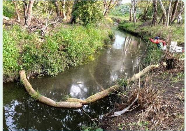
RMIT Aquatic Pollution Prevention Partnership (A3P) researcher collecting samples upstream of a pollution barrier sausage in Stony Creek
