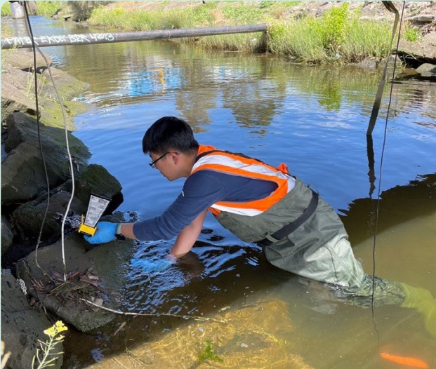
Monash University researcher installing water quality sensors in Stony Creek
