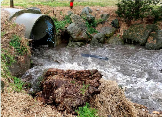
Stony Creek stormwater drain in high flow, with a black mesh sampling bag suspended midstream
