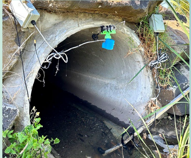
Above stream water sensor installed as part of the research trial in Stony Creek
