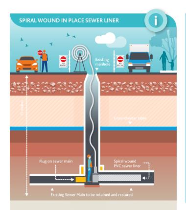
The technique we are using to upgrade the sewer is called 'Spiral Wound PVC'. This involves unwinding the relining material as a flat strip from a spool at the top of the manhole. The new plastic sleeve is wound into place, lining the inside of the existing sewer pipe. The gap between the existing pipe and new liner is then filled with cement (called grouting).
