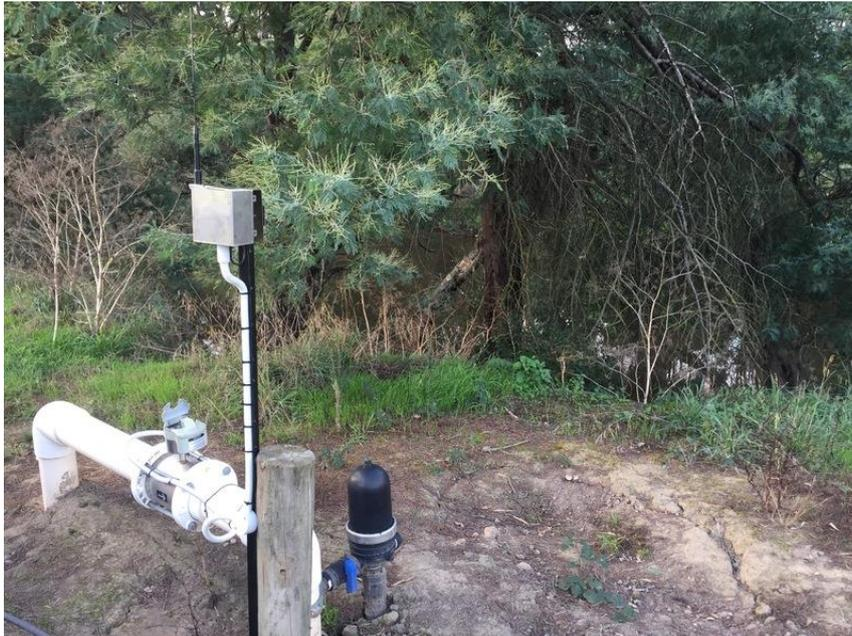
Figure 2: Full flowing pipe meter with Ajenti transmitter
