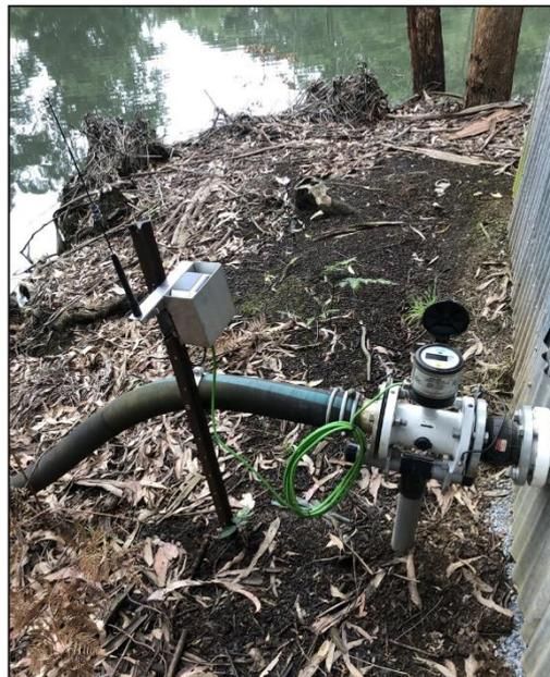
Figure 3: Siemens Mag8000 meter with Ajenti transmitter
