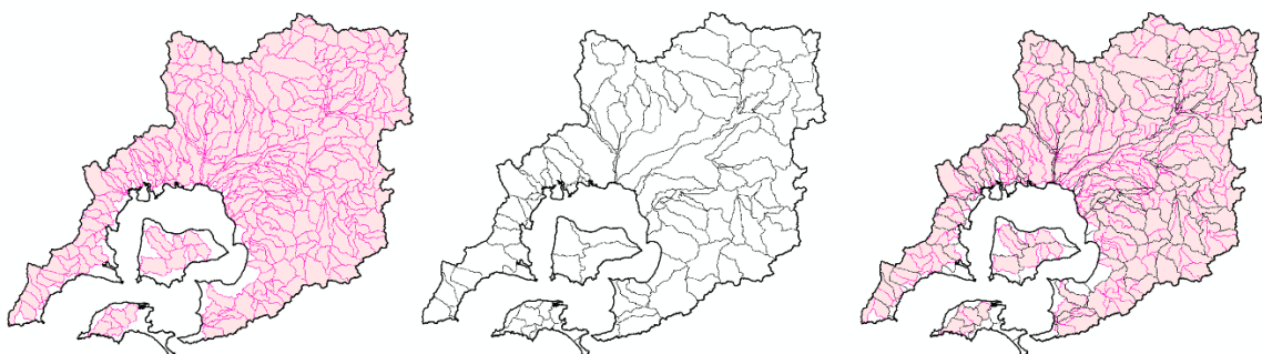
Figure 7 Revised finer resolution Westernport Model subcatchment delineation (left) compared to coarse resolution subcatchment delineation for the regional Port Phillip and Westernport Source model (middle). On the right is the two model subcatchment boundaries overlaid illustrating consistency between the two models
